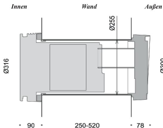
Alle Abmessungen in [mm]
